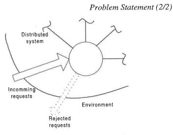
Imbalances of load causes situation where some nodes are below capacity while others are simultaneously overloaded
